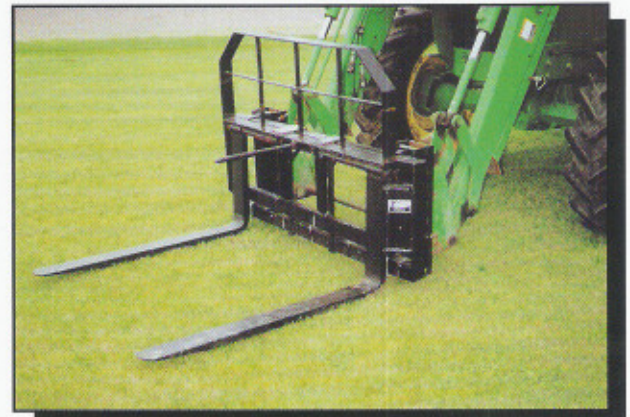
Tebben tractor loader fork assembly with universal mounting brackets.
