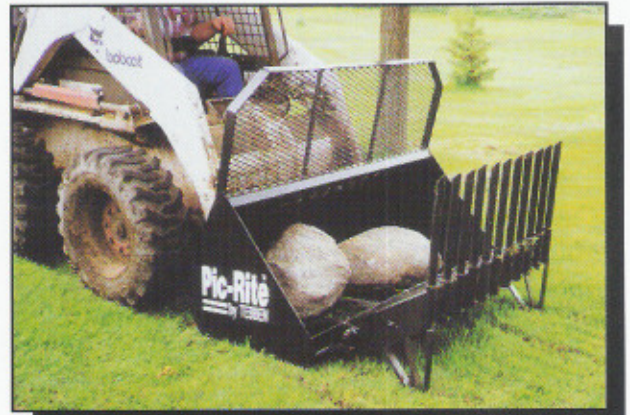
Tebben Pic-Rite™ rock picking bucket attachment digs rocks or skims under the surface for smaller rocks. Operates mechanically (no hydraulics needed) flips rocks into bucket by simply backing up.
