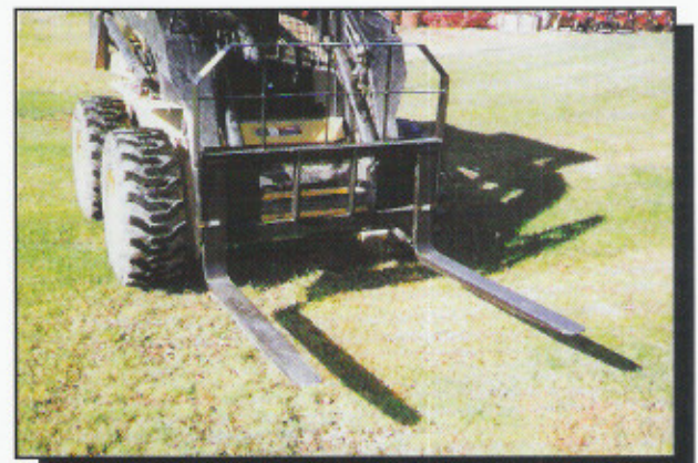
Tebben Skid Steer mount fork attachment with universal mount plate.
