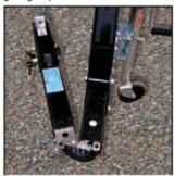
OPTIONAL GUIDE ROLLERS. Assists you when driving on in current or wind.
