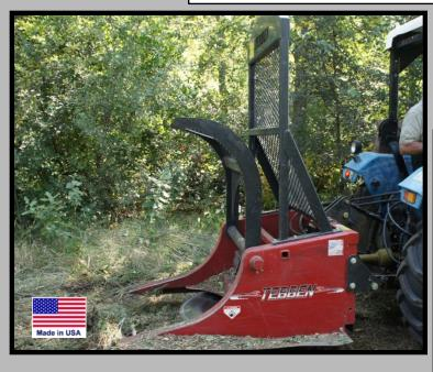
The Tebben Tree Saw is designed to cut down invasive trees easily, clean and fast.
